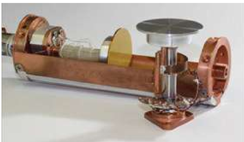
Fig. 6. Measuring chamber of the emissometer [30]: a) open chamber with the absorber part removed; b) diagram of the installation used to measure the emissivity
