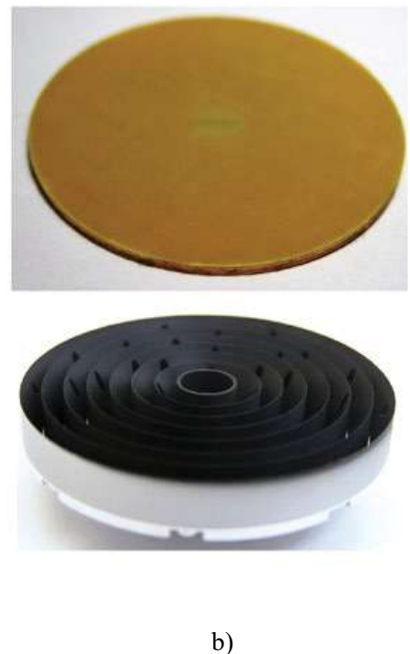
Fig. 7. Reference samples. Temperature dependence of their emission coefficient (a) and photograph (b) of the epoxy sample (upper picture) and the corrugated sample with V-shaped grooves [30]
